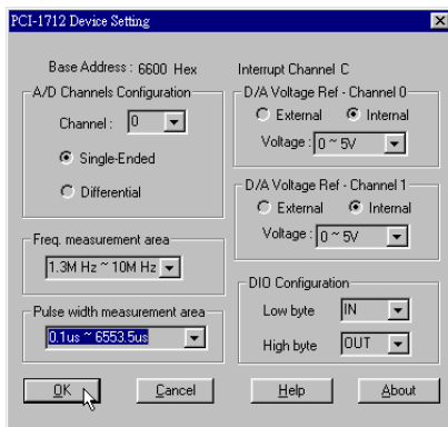
Figure 2-7: The Device Setting dialog box
