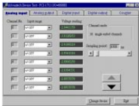
Fig. 2-11 Analog Input tab on the Device Test dialog box
